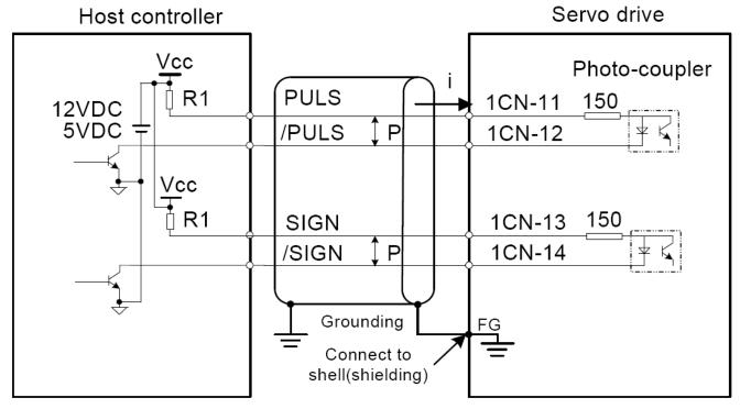
The correct current limiting resistor R1 should be used according to the current requirements of  $i = 10\sim15$ mA:
